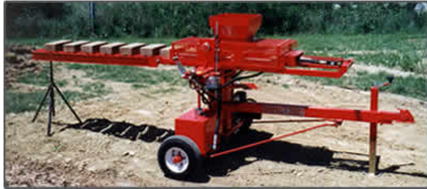
Lawrence Jetter of A.E.C.T. demonstrates this handy earth-block presser at the San Antonio classes.
